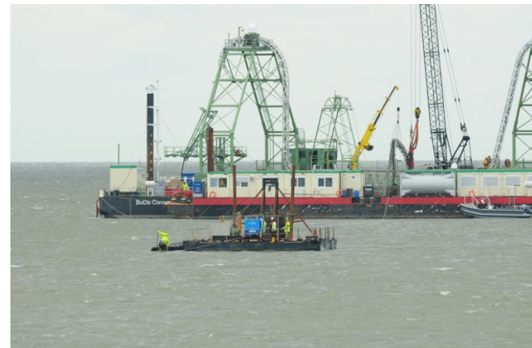
Anchor handling with very shallow draft anchor-ponton
