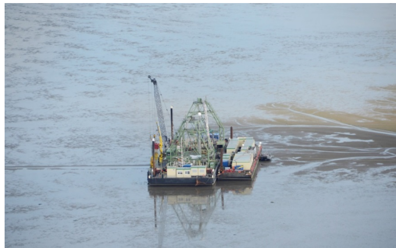
Installation barge with special designed Vibration Sword
